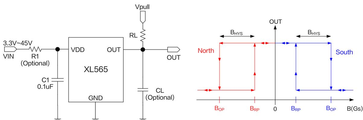
Figure1. XL565 Typical application schematic and output characteristic curve
