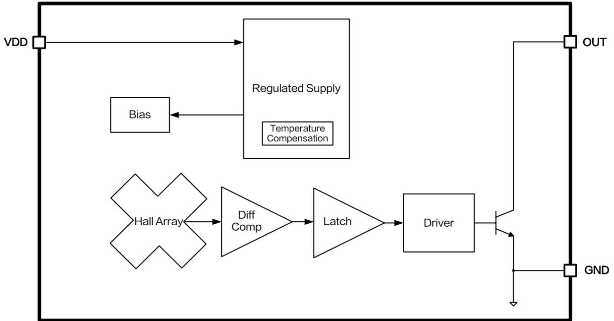
Figure3. Function Block Diagram of XL565
