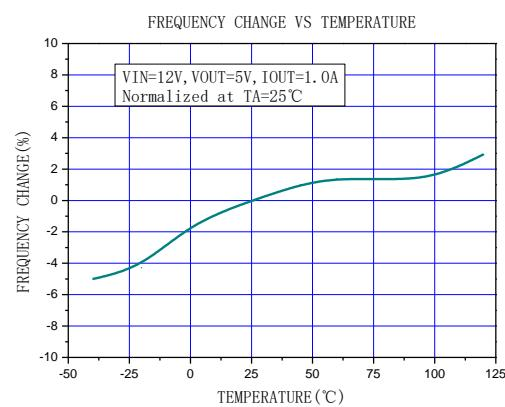
Figure10. Frequency change Curve
