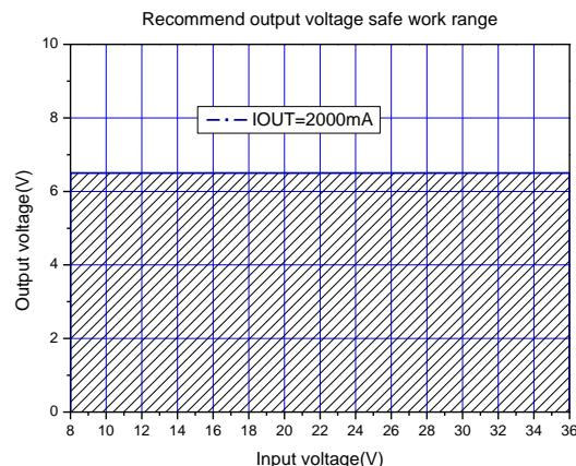
Figure15.Max output voltage(IOUT=2000mA)
