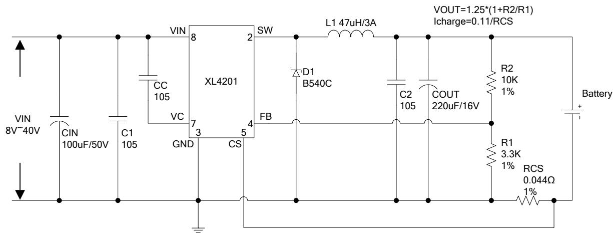
Figure4. XL4201 Typical Application Circuit (Li Battery Charger)
