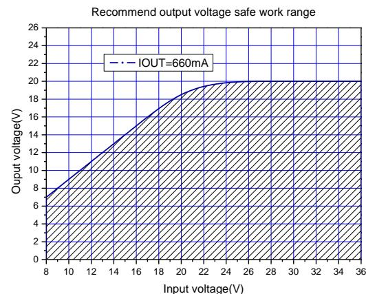
Figure13.Max output voltage(IOUT=660mA)
