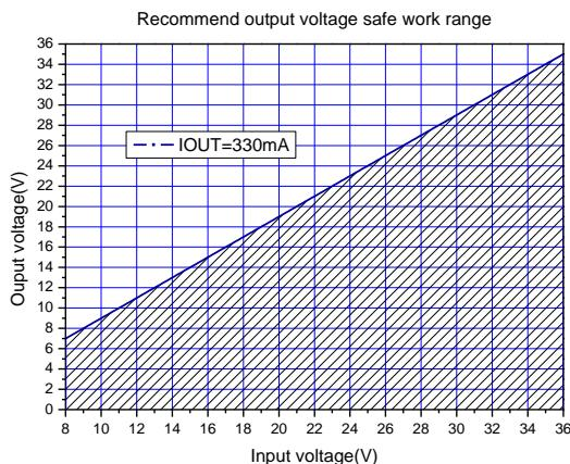
Figure12.Max output voltage(IOUT=330mA)
