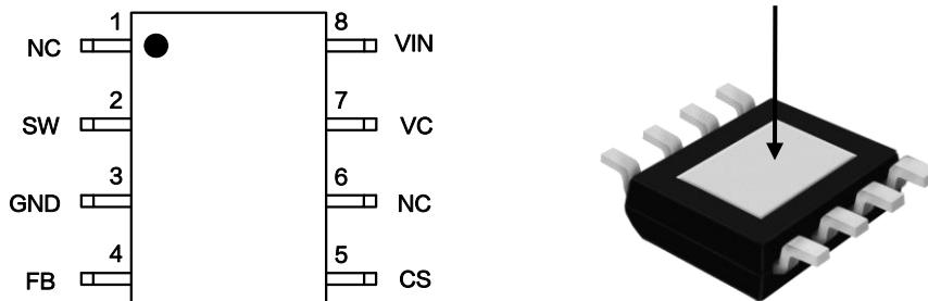
Figure2. Pin Configuration of XL4201 (Top View)
