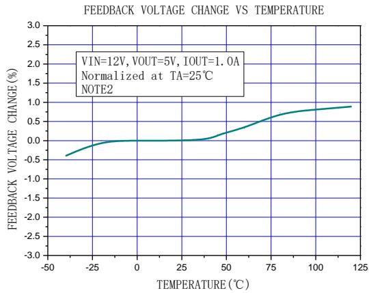
**Note2:** Internal temperature compensation circuitry is provided to compensate the PCB and external line loss in system application. When the junction temperature or the output power rise, the feedback voltage will be compensated. This function is provided to compensate the PCB and external line loss in system application.
