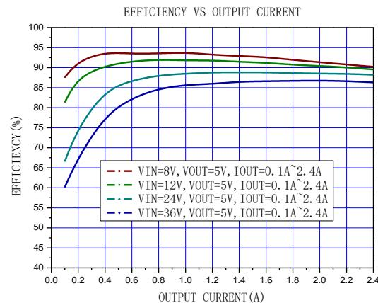
Figure8. Efficiency Curve
