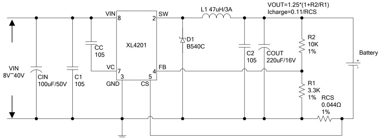
Figure6. XL4201 System Parameters Test Circuit (VIN=8V~40V, VOUT=5V/0.1A~2.5A)
