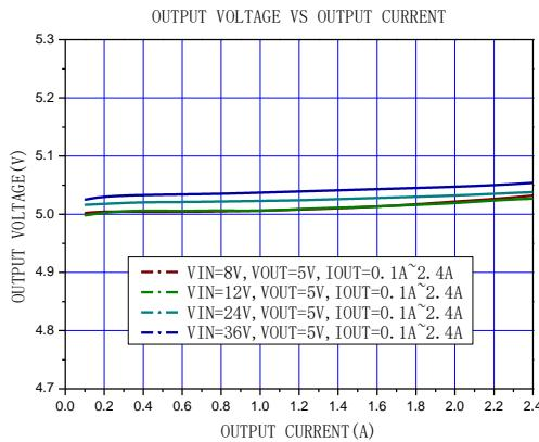
Figure9. Line&amp;Load regulation Curve
