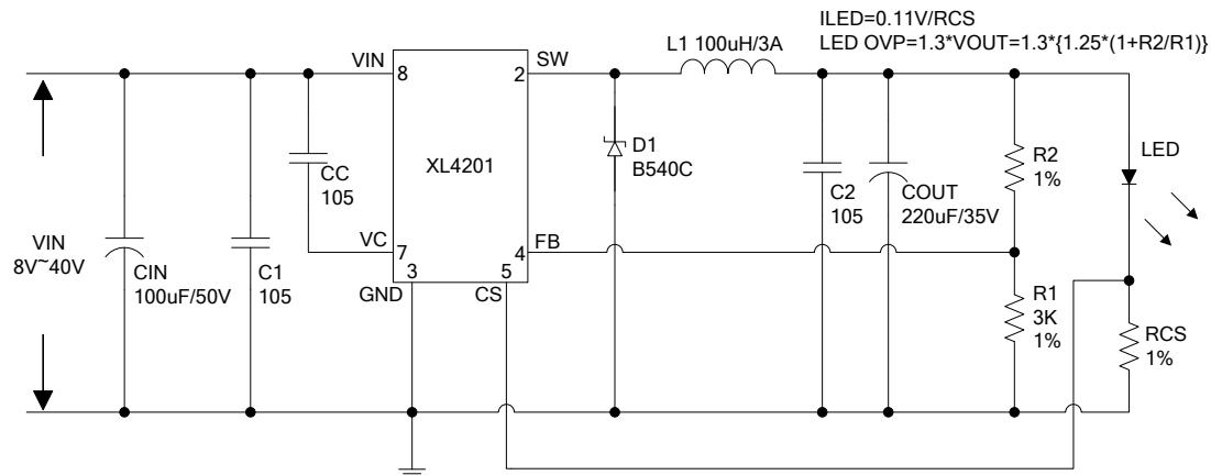
Figure5. XL4201 Typical Application Circuit(LED Constant Current Driver)
