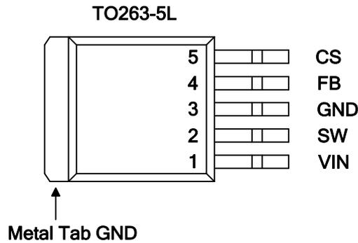
Figure2. Pin Configuration of XL4101 (Top View)
