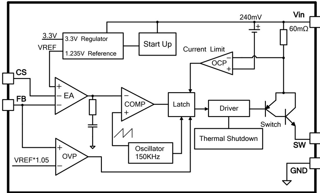
Figure3. Function Block Diagram of XL4101
