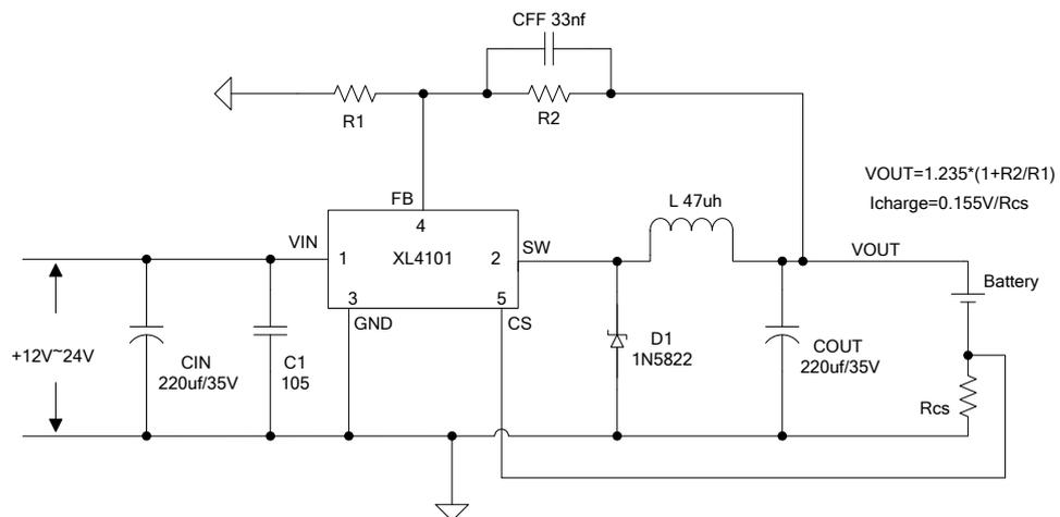
Figure4. XL4101 Typical Application Circuit (Li Battery Charger)
