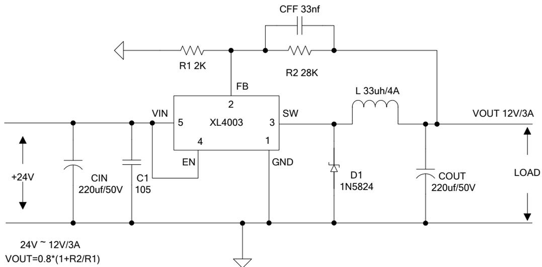
Figure6. XL4003 System Parameters Test Circuit (24V ~ 12V/3A)
