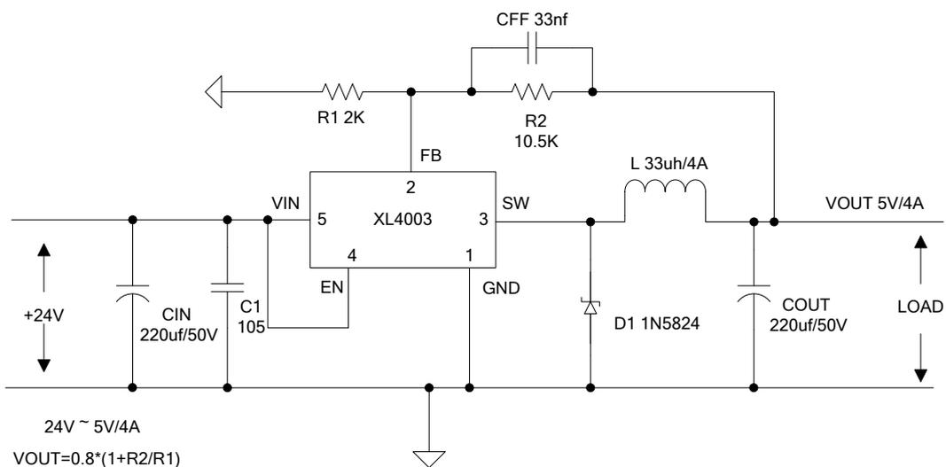
Figure7. XL4003 System Parameters Test Circuit (24V ~ 5V/4A)
