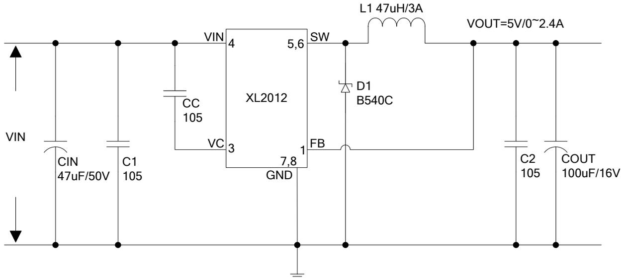
Figure5. XL2012 System Parameters Test Circuit (VIN=8V~40V, VOUT=5V/2.4A)
